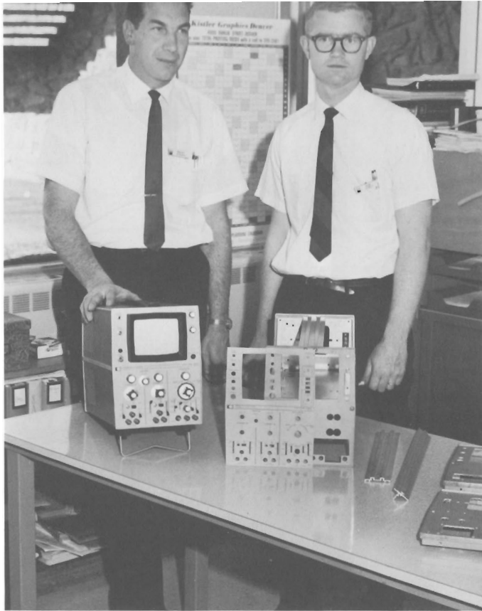
Design engineers Ralph Jensen, left, and Bob Jones of Colorado Springs exhibit cabinet and castings of new 1200 series low-frequency scopes. Modular design permits several instruments to use same cabinet, CRT and power supplies. Same main frame can be used in future instruments. Since many modules are common to various models, production quantities are large enough to justify automatic testing as shown above.
