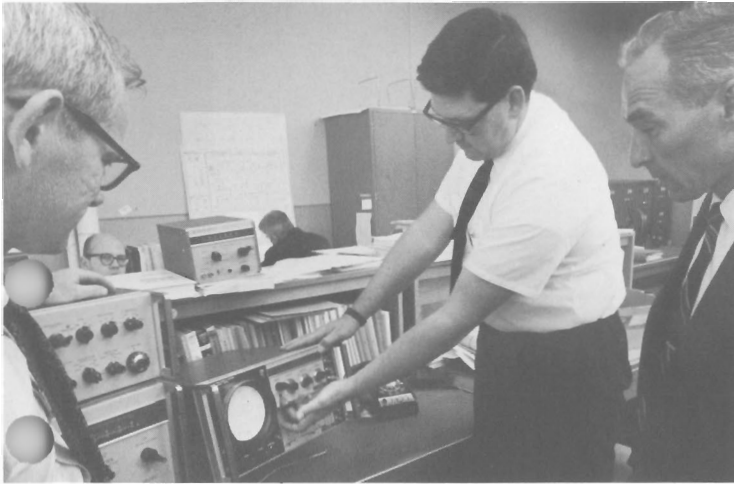
Early establishment of service procedures for this new second-generation HP spectrum analyzer is the goal of the team shown here—Bill Downs (left) and Jim Shea, Microwave service engineers, and Ray White of Corporate Service Center. Specifically, they are discussing data on calibration of the instrument for inclusion in operating manual.
